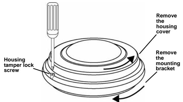
Figure 2 Remove the housing cover and mounting bracket
