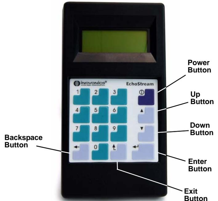
**Figure 3** EE4016SK Survey Receiver
