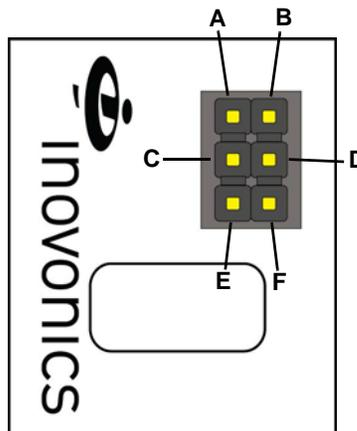
Figure 2 OEM connector pinout
