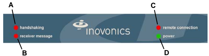
Figure 2 RDL8500 remote data logger front panel
