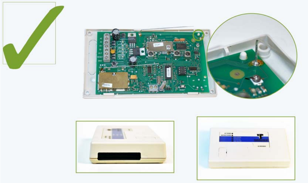
Figure 7 Properly seated board and housing cover.
