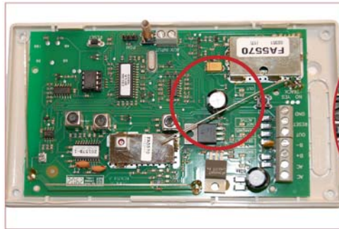
Figure 4 FA antenna obstructed by board component.
