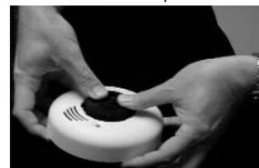
Figure 5: Removing the sensor from the detector body
