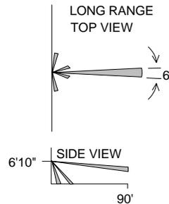
Long range: Designed to look down aisles, up or down stairwells or for perimeter protection. Range of 90 feet for long range zone. Three short-range lookdown zones protect the area near the Sharpshooter.
