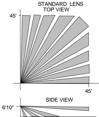
Standard: The standard lens covers a 90° field, and has a 45-foot range. It has lookdown zones of 60°, 30°, 15° and 4°.
