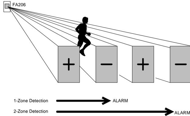
The one-zone detection option tells the Sharpshooter that changes in any adjacent wedges should cause an alarm. This setting is required for long-range lenses and curtain lenses. In standard lenses, however, one-zone detection makes the unit very sensitive to minor temperature variations in the environment, and can result in false alarms.
