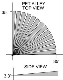
Pet Alley: The pet alley lens covers a 90° field, and has a 35-foot range. Recommended mounting height is 3.3'.
