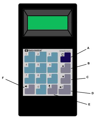
Figure 8 Survey receiver keypad.
