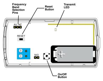
Figure 3 EN1210SK survey transmitter
