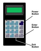
Figure 1 EN4016SK survey receiver
