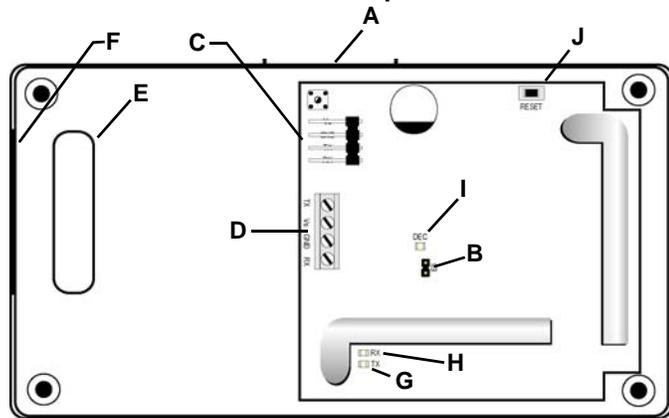
Figure 2 EE4200H-HSG serial receiver components
