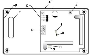
Figure 2 EE4200H-HSG serial receiver components
