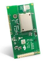
The EN1941XS one-way serial data RF module provides reliable low-cost, low-power serial wireless communication for integrators. The EN1941XS is a universal one way RF module that allows for the transmission of up to 50 bytes of user defined serial data. This module connects to a serial interface to transmit variable data such as temperature, humidity, pressure, or liquid levels to a head end application controller.
