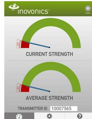
**Figure 9** You will need a repeater if both needles are in the red
