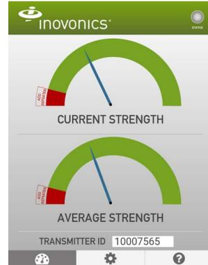
**Figure 8** If the signal strength is green, you don't need a repeater
