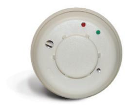
The wireless smoke detector features an onboard sounder, a smoke sensor, an LED indicator and local test capability to allow the user total visibility of its functionality. It is self-monitoring, alerting the user when sensor maintenance is needed or batteries are low, and automatically supervising the radio link.
