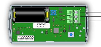
Black wire to terminal B on register Green wire to terminal G on register Red wire to terminal R on register
