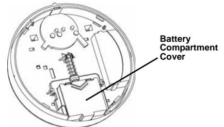
Figure 3 Remove the EE1243 battery compartment cover
