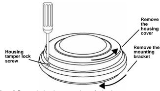
Figure 2 Remove the housing cover and mounting bracket
