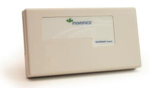
The security only serial receiver is a wireless gateway between EchoStream one-way security transmitters and a head end application using an RS-232 serial interface.
