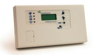
The Inovonics 16 zone multi-condition receiver with relay outputs programs and supervises up to 16 single or multiple condition transmitters. This receiver includes Form C relays, allowing connection to any hardwire panel or stand-alone wireless application.
