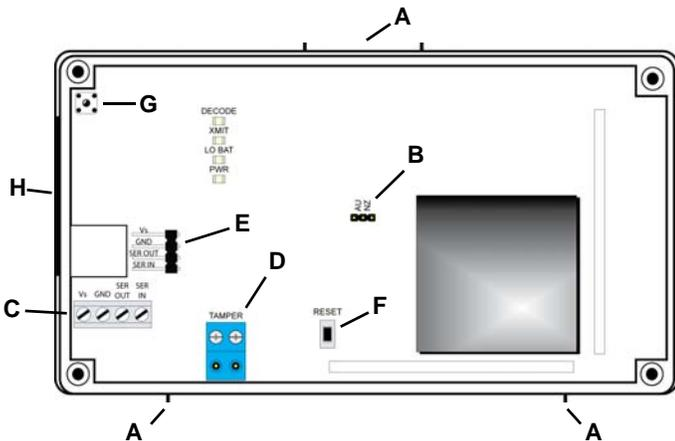
**Figure 3** EN6040-T network coordinator internal components
