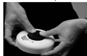
Figure 5: Removing the sensor from the detector body
