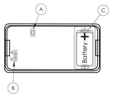
A Reset button B Frequency band selection pins C Battery
