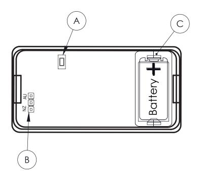
A Reset button **B** Frequency band selection pins **C** Battery
