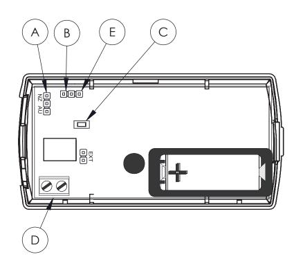
A Frequency band selection pins B Programming header pins C Reset button D Probe terminal block E Programming header pin 1
