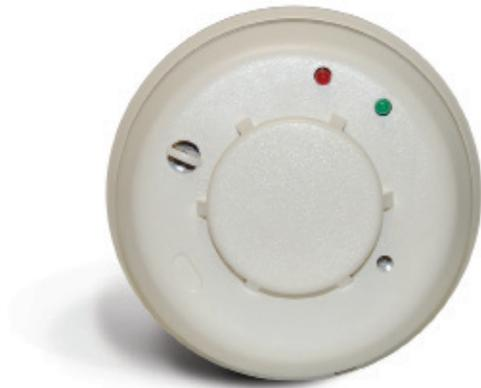
The wireless smoke detector features an onboard sounder, a smoke sensor, an LED indicator and local test capability to allow the user total visibility of its functionality. It is self-monitoring, alerting the user when sensor maintenance is needed or batteries are low, and automatically supervising the radio link. The EN1244-60 wireless smoke detector sends check-in messages every 60 minutes to allow for use in a UL 2560 certified system.
