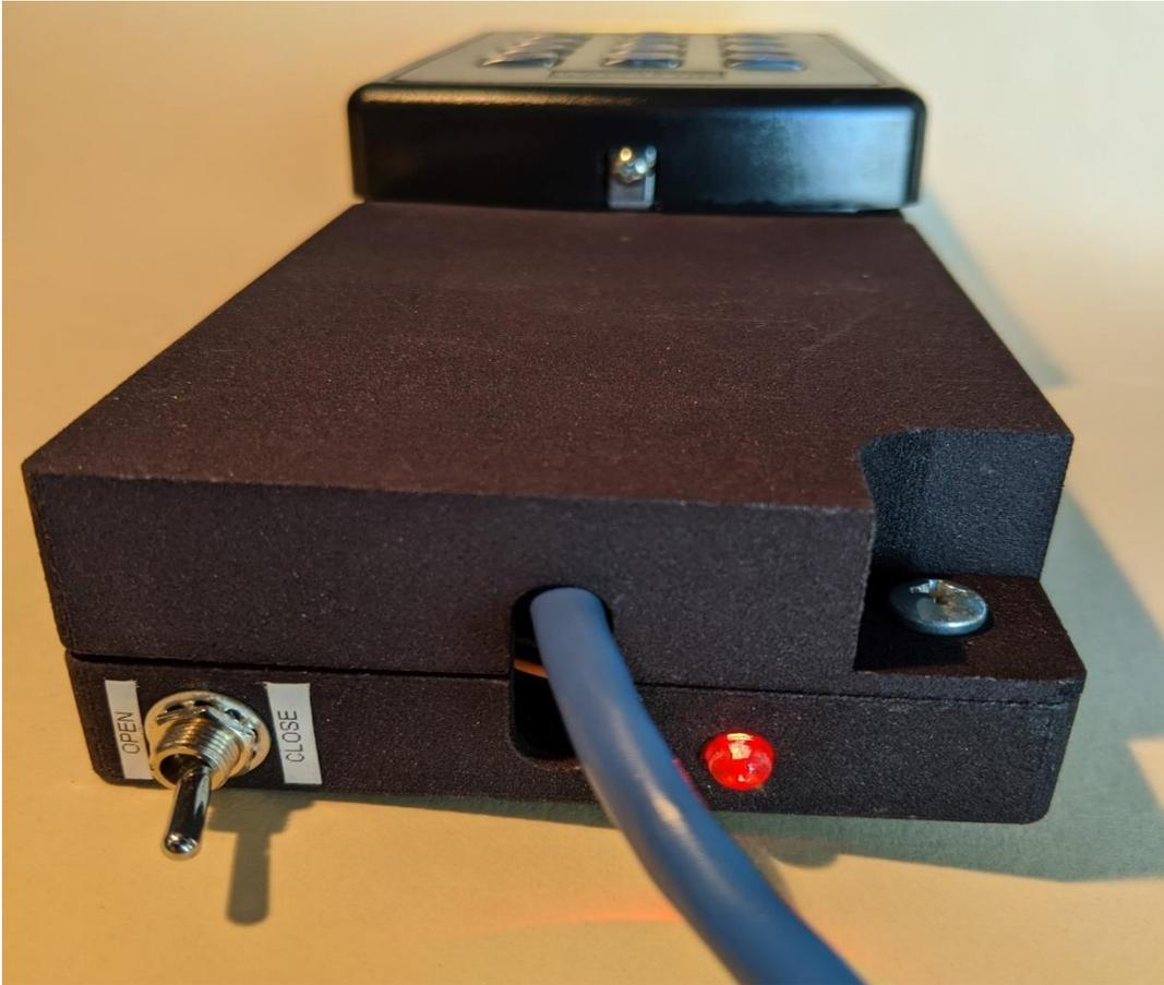
At the bottom of the wall unit, you'll notice a test door switch and a test lock LED. The test door "toggle" switch can be used to simulate a door opening and closing. The test lock LED will glow red when the lock is activated. The hole located between the toggle switch and the LED is available to run the power and Ethernet cable.
