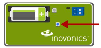
4. Press the reset button to initialize the transmitter.
